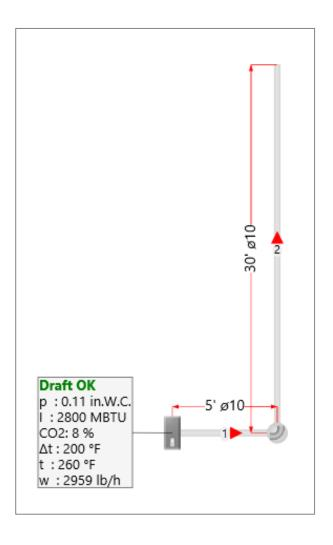
35', single elbow, max. back pressure 0.25 in.W.C.
